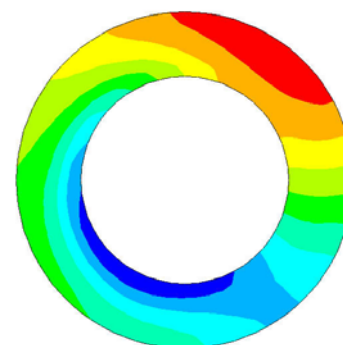
Figure 10: Oil-film thickness distribution on the thrust surface (The darker the blue the smaller the oil-film thickness).
