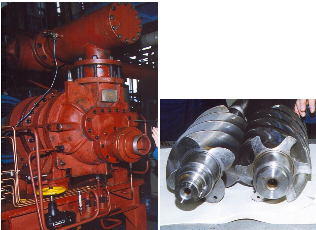
Fig. 2 Compressor and prototype rotors in the industrial premises
