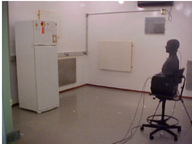
Figure 2 – General test room view with refrigerator and head and torso simulator.
