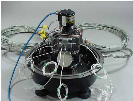
Fig. 4: Instrumented compressor general view.
