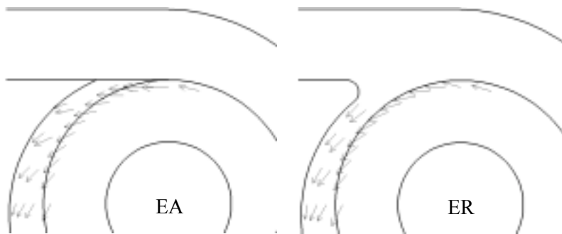
Fig.14-a Distribution of velocity vector, Component parallel to the diffuser wall (Flow coeff.=0.19)
