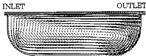
Figure 6. Flow Pattern in Labyrinth Groove
