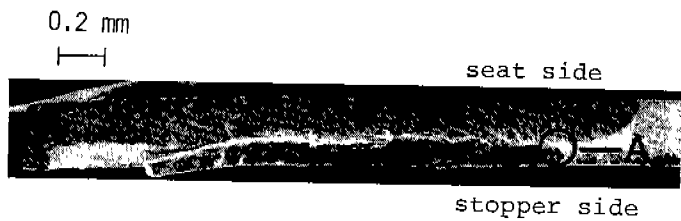
Fig. 9 Allover view of impact fatigue failure surface
