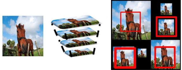
Figure 5. We use the image patchwork technique to efficiently implement scale and position search in DCNN training: an image pyramid is unfolded into a image ‘patchwork’, where sliding a fixed-size window amounts to search over multiple positions and scales. The maximum of the classifier’s score on all such windows is efficiently gathered by max-pooling the DCNN’s top-layer responses, and is used to accommodate scale and position changes during both training and testing.
