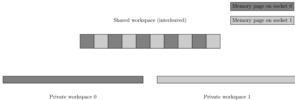
Figure 3.2: Illustration of the adaptation of the ALGTIME factorization phase for NUMA architectures on an example with two threads under \mathcal{L}_{th} , each mapped on a core of different sockets, and both working together above \mathcal{L}_{th} .
