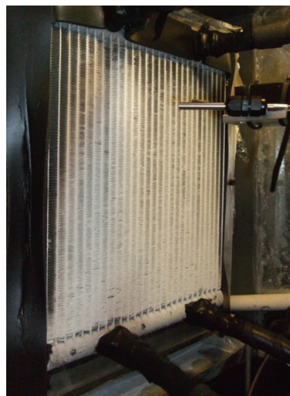
Figure 1: Schematic of the air wind tunnel for low temperature frosting experiments (left) and Image of the microchannel coil under frosting inside the low temperature air wind tunnel (right).
