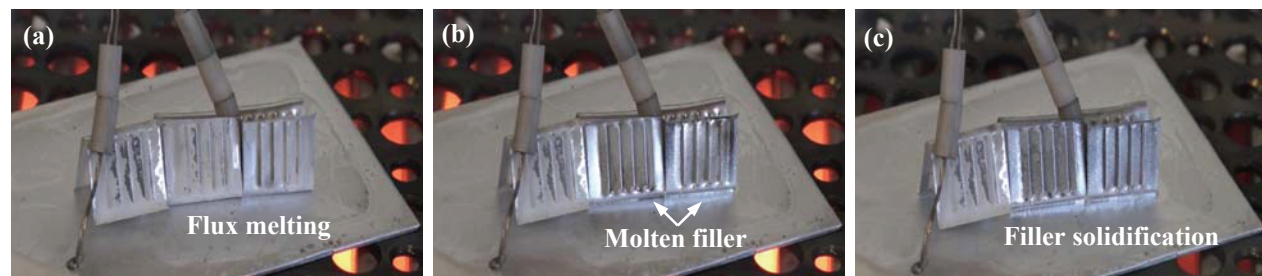
Figure 4: In-situ monitoring of fin/tube joint formation (a) flux melting; (b) joint formation; (c) solidification
