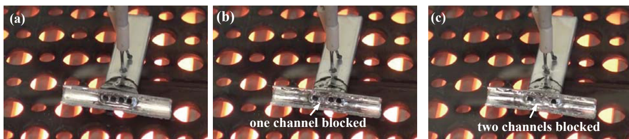
Figure 10: In-situ monitoring of liquid filler metal blocking microchannels using glass furnace: (a) molten filler formed joint between header and tube; (b)&(c) microchannels being blocked by molten filler
