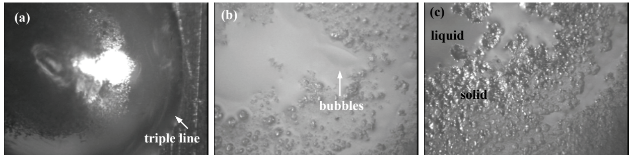
Figure 5 A sequence of frames extracted from a real-time monitoring of molten filler spreading using hot stage microscopy (a) spreading; (b) liquid surface features bubbles; (c) solidification.
