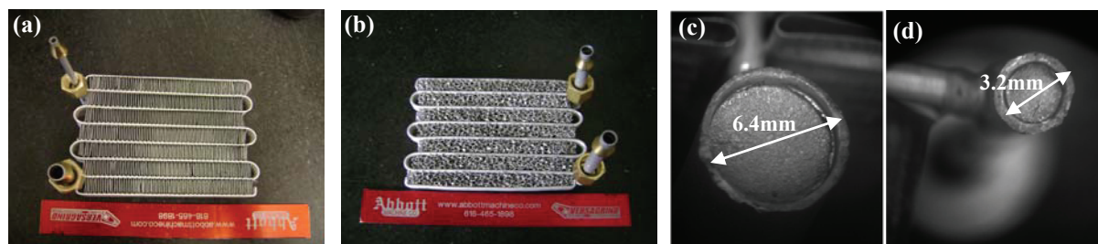
Figure 8 Serpentine condenser fabricated using CAB brazing (a) louver fin condenser ; (b) foam condenser; (c) 6.4mm OD header/tube joint; (d) 3.2mm OD header/tube joint.
