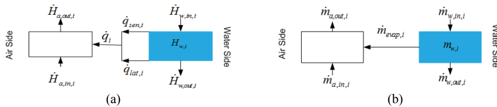
Figure 2: (a) Energy Balance between Neighbored Water and Air Control Volumes and (b) Mass Balance between Neighbored Water and Air Control Volumes
