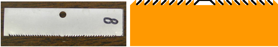
Figure 6: (a) The aluminium saw tooth DES designed for enhanced contact with louver. (b) The schematic showing saw tooth of DES meshed with louver spaces. The saw tooth pitch was of the same magnitude as the louver pitch
