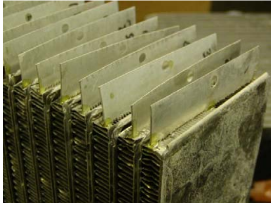
Figure 7: Picture shows the saw toothed DES mounted on the heat exchanger.
