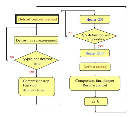
Figure 6: Defrosting Control Method
