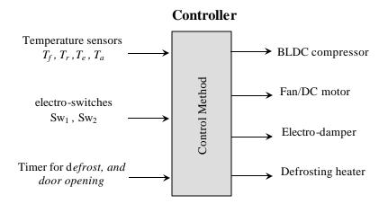
Figure 4: Control methods for variable frequency refrigerators/freezers.
