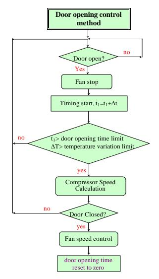
Figure 7: Door Opening Control Method.
