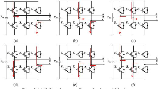
Figure 2: (a)-(f) Control sequence diagram for six-step driving inverter.
