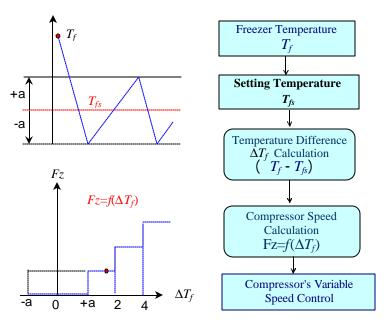
Figure 5: Frozen food storage temperature control flowchart.
