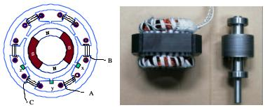
Figure 1: Inner structure and photo of four-pole brush-less DC motor.
