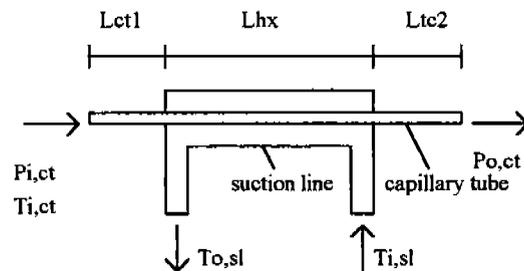
Figure 2: Longitudinal view of concentric-tubes HX.
