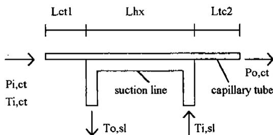
Figure 1: Longitudinal view of lateral heat exchanger.
