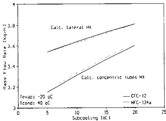
Figure 3 - Influence of sub cooling on the mass flow rate for two heat exchanger configurations and for CFC-12 and HFC-134a.
