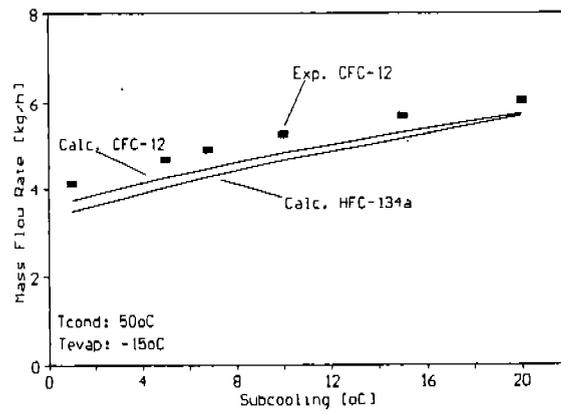
Figure 4 - Comparison between experimental and numerical results for an adiabatic capillary tube.
