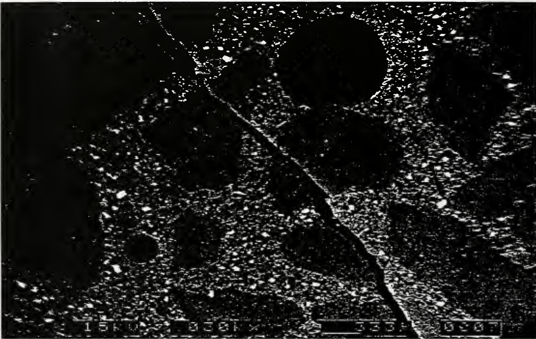
Figure 7.75 BEI micrograph of flexural tensile crack in quartzite mortar, magnification 30 \times , mixture proportion 37_52_10, aggregate size #16~#30.
