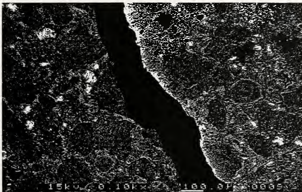
Figure 7.70 BEI micrograph of flexural tensile crack in dolomite mortar, magnification 100 \times , mixture proportion 37_52_10, aggregate size #50~#100.
