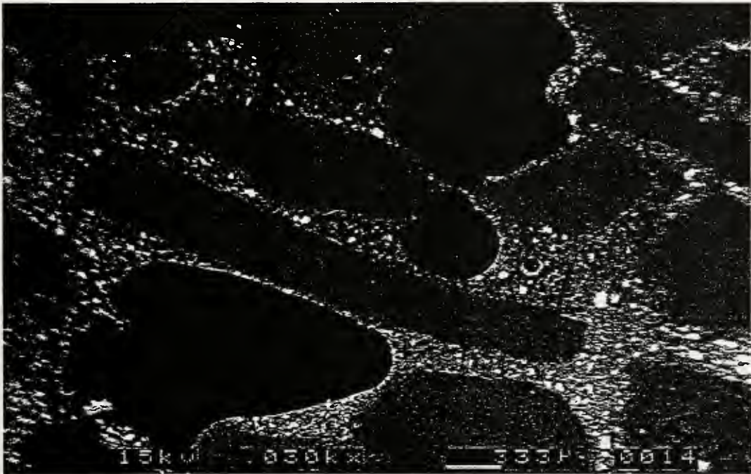
Figure 5.13 BEI Micrograph of Large Pores in Dolomite Mortar, magnification 30 \times , mixture proportion 65_42_00, aggregate size #8-#16.
