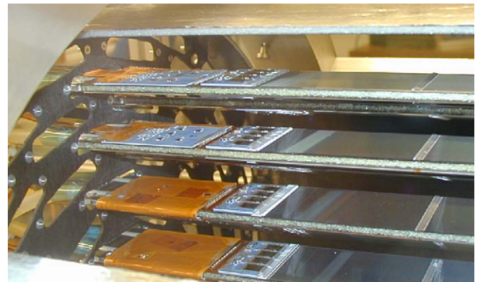
Fig. 1. Photograph of supermodules installed in the barrel. The outer bulkhead is on the left.
