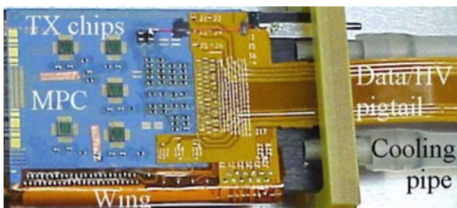
Fig. 20. A photograph of the top side of the beryllia mini-port card.
