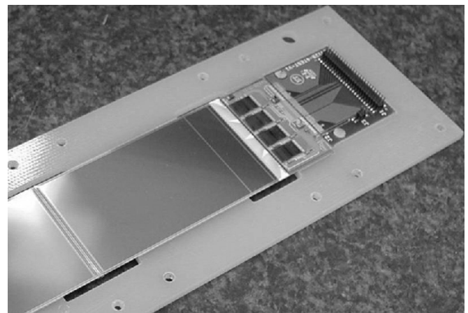
Fig. 7. Picture of module. Two silicon sensors are wire bonded and held by a G10 frame. One side of the sensor is bonded to a pitch adapter which connects to the SVX4 chips on hybrid.
