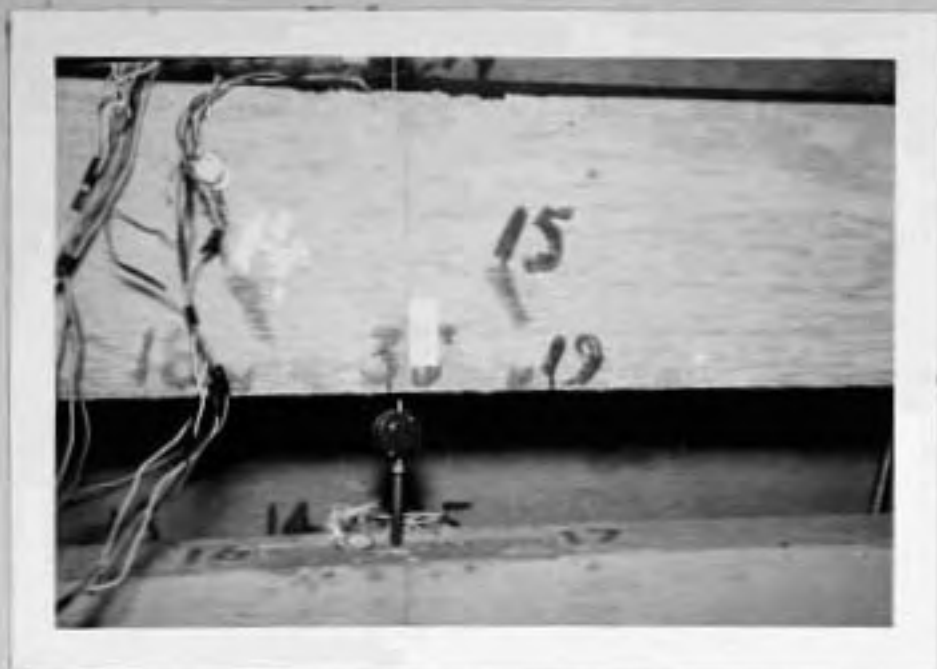
FIG. 20 CAMBER DETERMINATION, COPPER WIRE AT CENTERLINE
