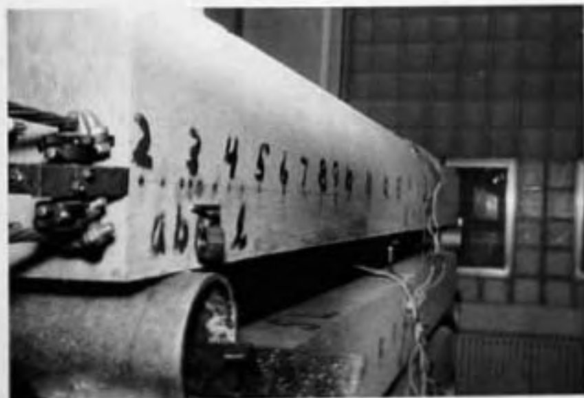
FIG. 19 CAMBER DETERMINATION, SUSPENSION OF COPPER WIRE
