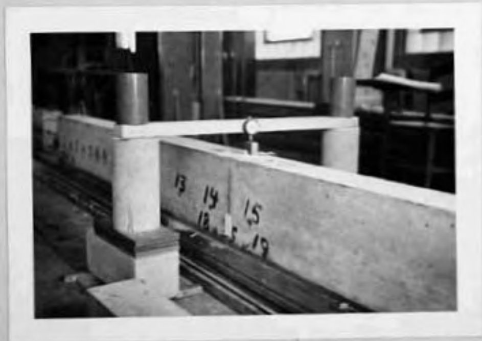
FIG. 21 CAMBER DETERMINATION, USE OF DIAL GAGE
