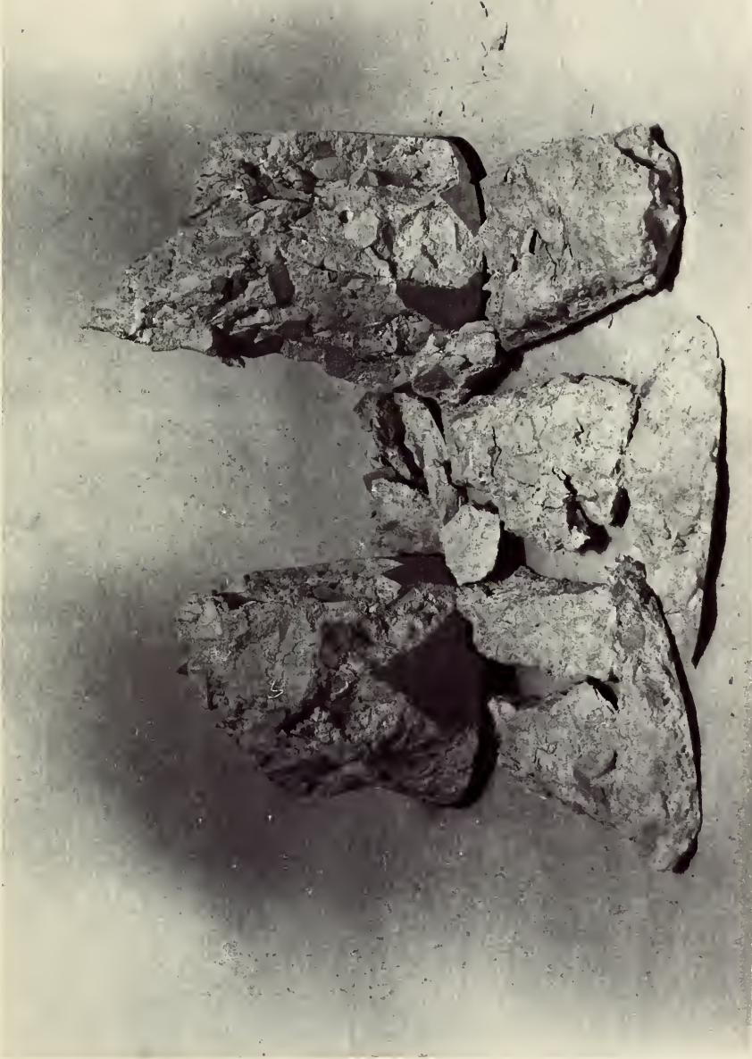
FIGURE 8. TYPICAL FAILURE FOR 0.70 w/c A-1 AGGREGATE CONCRETE
