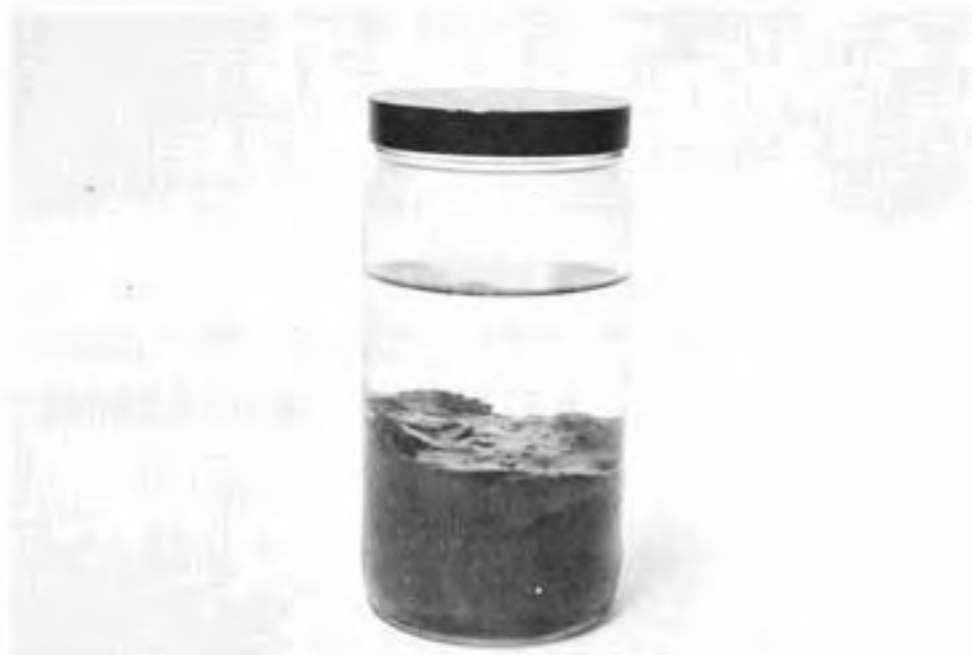
FIGURE 10. CANNELTON SHALE AFTER 15 MINUTES OF IMMERSION IN WATER.
