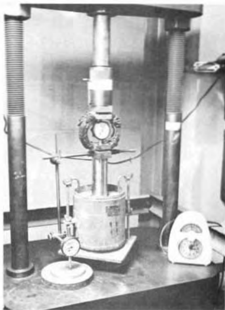
FIGURE 15. LOADING DEVICE FOR CBR TEST.
