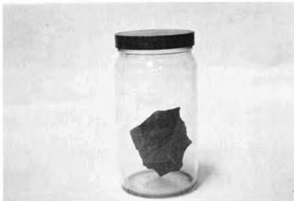
FIGURE 9. CANNELTON SHALE BEFORE IMMERSION IN WATER.
