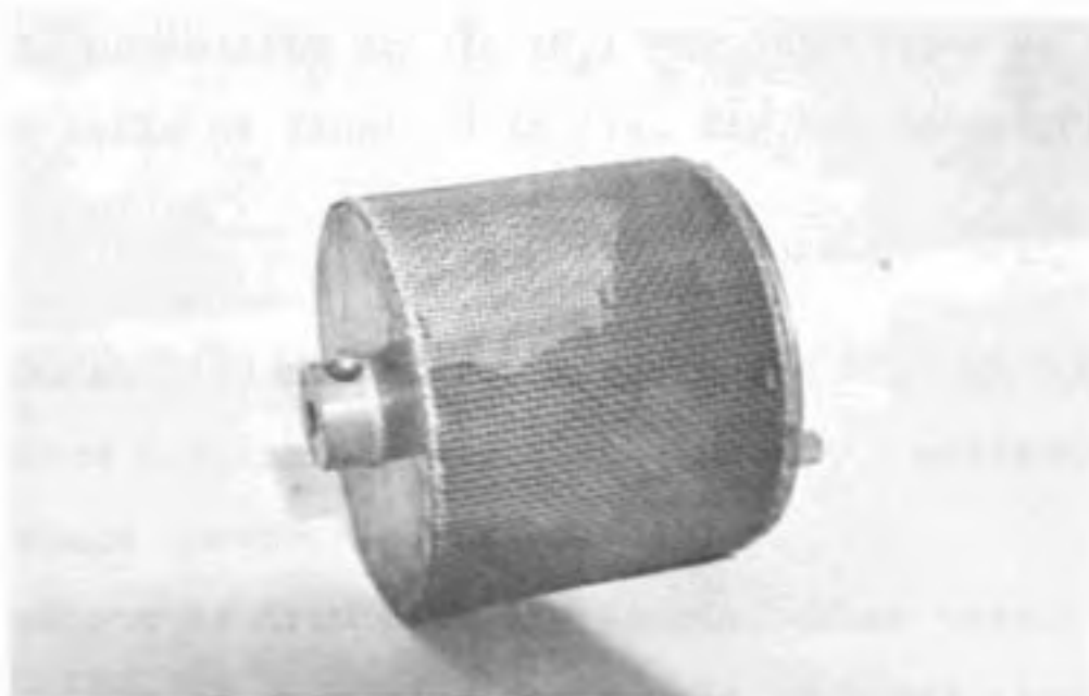
FIGURE 13. TEST DRUM IN SLAKE DURABILITY APPARATUS.
