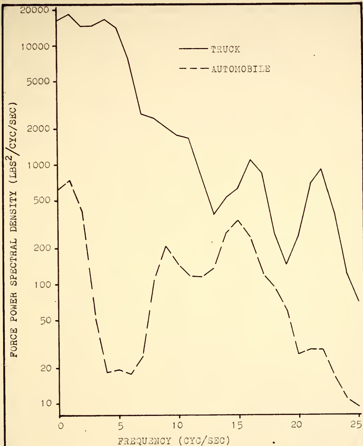
FIGURE 61 COMPARISON OF EXPERIMENTAL RESULTS FOR AN AUTOMOBILE AND THE TEST TRUCK
