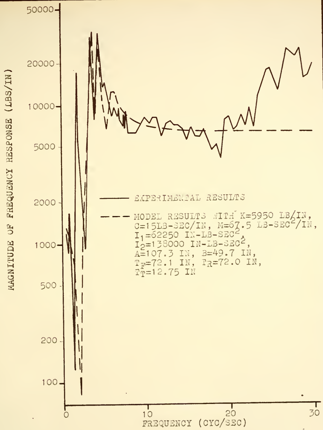
FIGURE 41 COMPARISON OF THE MODEL FREQUENCY RESPONSE WITH EXPERIMENTAL RESULTS
