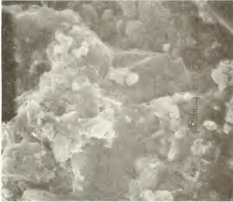
Figure 24. SEM Micrograph. Low Porosity Cement Paste, W:C 0.22, at 36 Hours. (a) ( x 3000 ).
