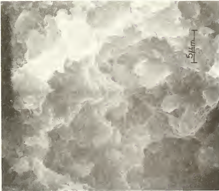
Figure 25. SEM Micrograph. Low Porosity Cement Paste, W:C 0.22, at 36 Hours. (b) ( x 3000).
