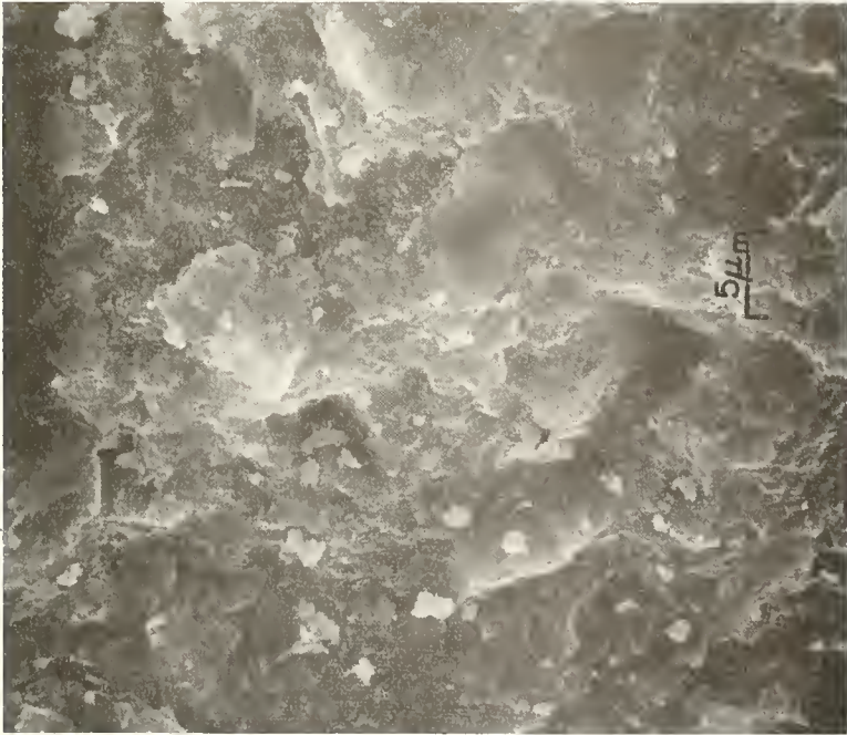
Figure 37. SEM Micrograph. Low Porosity Cement Paste, W:C 0.24, at 90 Days. ( x 2000).
