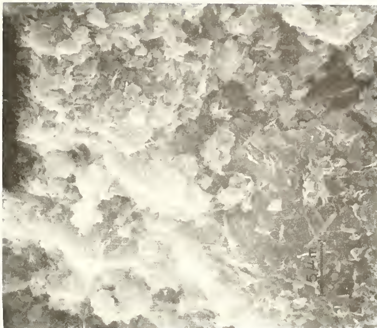
Figure 16. SEM Micrograph. Low Porosity Cement Paste, W:C 0.22, at 15 Hours. ( x 3000).
