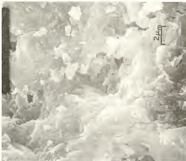
Figure 29. SEM Micrograph. Low Porosity Cement Paste, W:C 0.24, at 7 Days. (a) ( x 5000).
