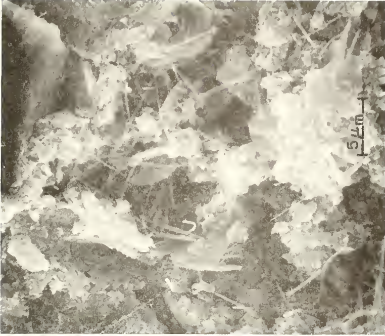
Figure 36. SEM Micrograph. Low Porosity Cement Paste, W:C 0.24, at 28 Days. Detail. ( x 3000).
