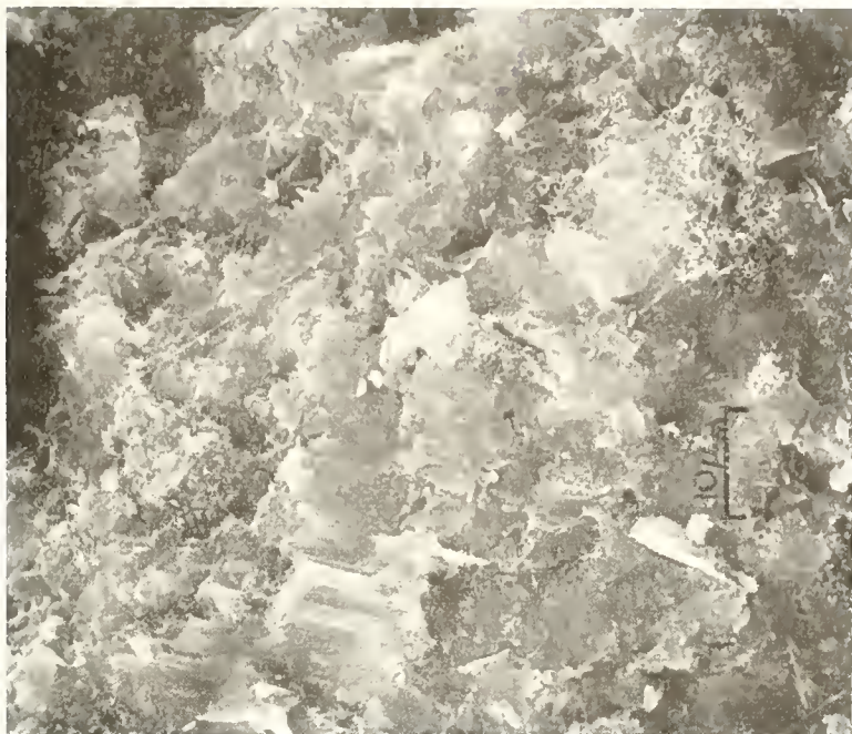
Figure 42. SEM Micrograph. Micro-structure of Bottle Hydrated Low Porosity Cement Paste, W:C 10, at 140 Days. ( x 1500 ).
