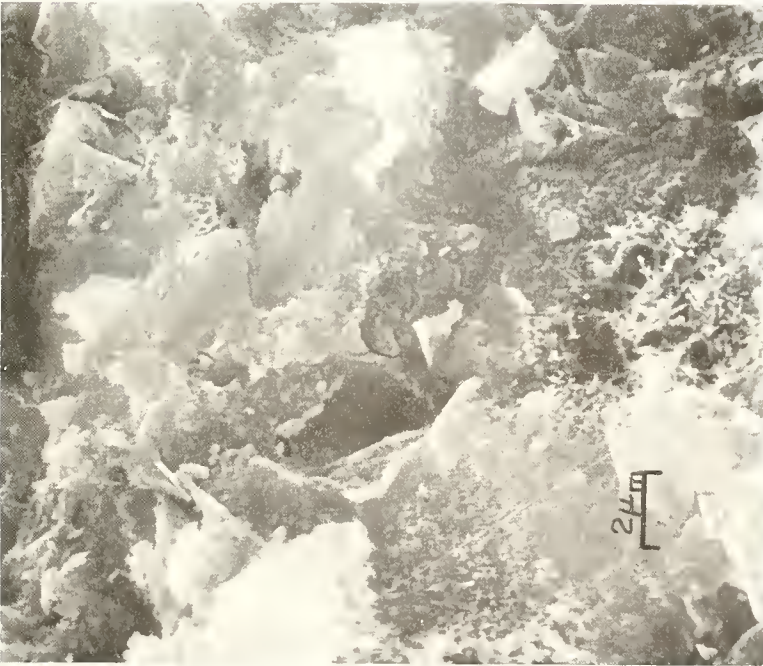
Figure 43. SEM Micrograph. Bottle Hydrated Low Porosity Cement Paste, W:C 10, at 140 Days. ( x 5000).
