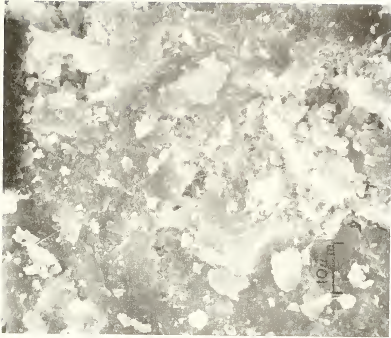
Figure 40. SEM Micrograph. Microstructure of Low Porosity Cement Paste, W:C 0.24, at 90 Days. ( x 1500).
