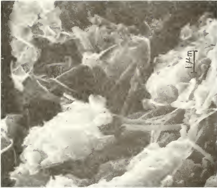
Figure 18. SEM Micrograph. Low Porosity Cement Paste, W:C 0.22, at 15 Hours. ( x 10000).
