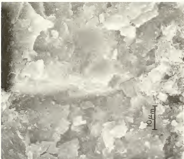
Figure 31. SEM Micrograph. Microstructure of Low Porosity Cement Paste, W:C 0.24, at 28 Days. ( x 1500).
