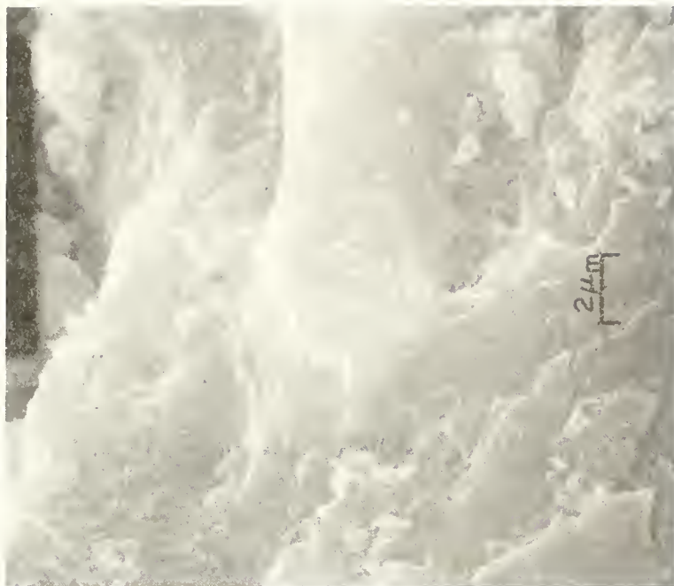
Figure 30. SEM Micrograph. Low Porosity Cement Paste, W:C 0.24, at 7 Days. (b) ( x 5000).
