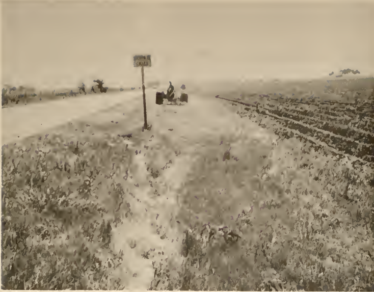
Fig. 9. Portion of SR 28 test plots photographed July 31, 1973. Except for growth of wild carrot (foreground), this plot required only a single midseason mowing.
