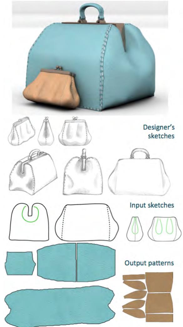
Fig. 15. Top: Doctor bag and leather purse designed with our system. Middle: designer's sketches exhibiting design folds which are intended to remain permanently on the product and the sketches given as input to our system. Bottom: the patterns we output. Note that we did not use symmetry for these examples: therefore, neither the input sketches nor the resulting shapes or patterns are fully symmetric.
