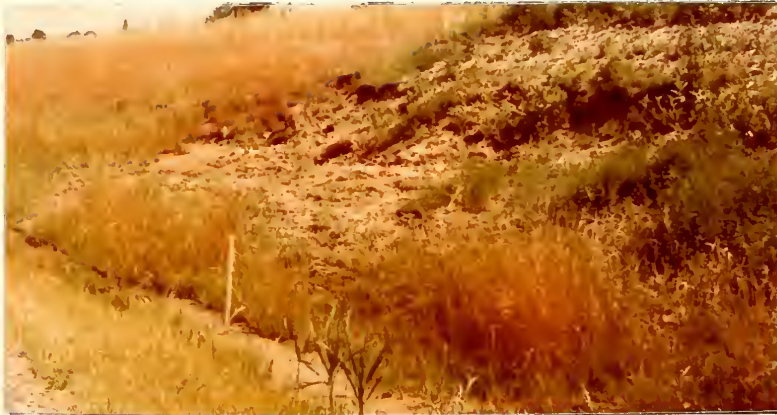
P.10 Hy. 38 & I-65. Elevated Island. Seeded to left & right. Sodded to experimental selections in center & background.
