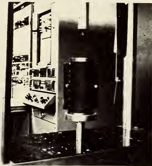
FIGURE 21 VIBRATORY COMPACTION OF MIXES
