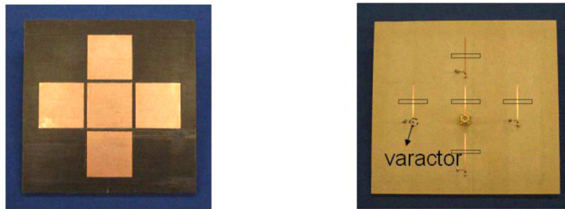
Fig.2 Fabricated parasitic patch array
