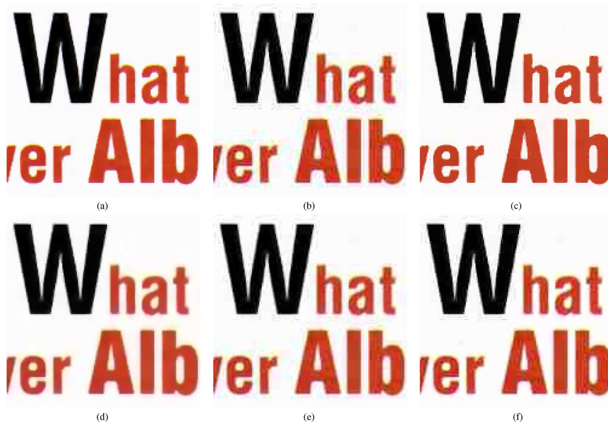
Fig. 15. Text region from Image 3. (a) Original. (b) Conventional JPEG decoding (c) The proposed algorithm. (d) Algorithm I [11]. (e) Algorithm II [34]. (f) Algorithm III [3]. For (f), only the text in red is decoded by the text decoding scheme of Algorithm III. The portion of the document corresponding to the letter “W” is decoded as picture by Algorithm III.
