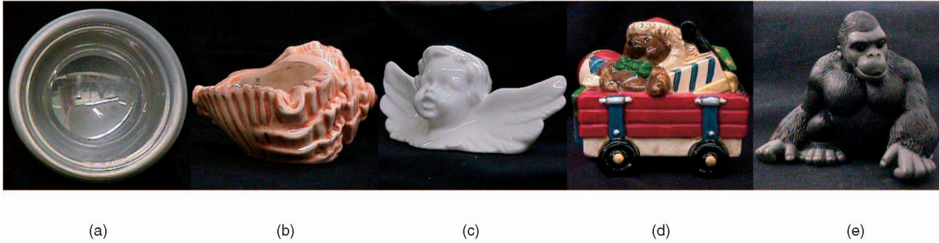
Fig. 16. Objects used in the experiment. (a) A stainless steel bowl. (b) and (c) Ceramic glazed seashell and angel figurines. (d) A tray figurine made of multiple materials, including specular, Lambertian, and highly absorptive surfaces. (e) A gorilla figurine made of black plastic. All objects have surface materials that are optically challenging.
