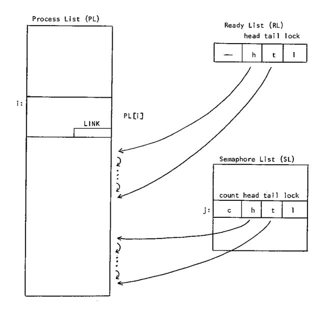
FIGURE 1: Process manager data structures.
