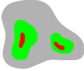
Figure 5: Multi-scale analysis illustration. Green: map thresholded at u(1) , red: map thresholded at u(2) > u(1) , and gray: regions below u(1) and u(2) . A probability is assigned to each region above the thresholds u_1 and u_2 .
