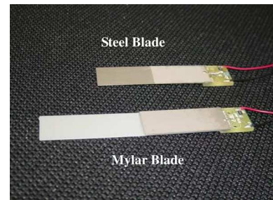
Fig. 4. Two piezoelectric fans (mylar and steel blades) tested to characterize the influence of operating parameters.
