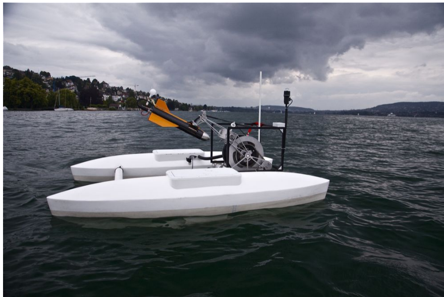
Figure 3.13: The autonomous surface vessel, named Lizhbeth, during one of its survey environment: pre-alpine Lake Zurich, Switzerland. The sensor was not installed at the time of the photograph.
