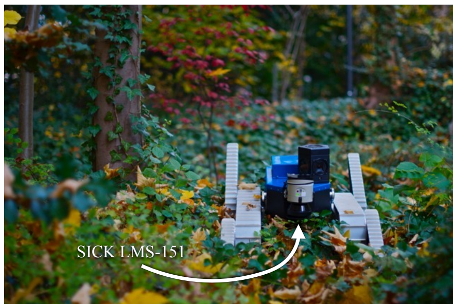
Figure 3.1: Photograph of NiftiBot, the main platform used for Search & Rescue demonstrations in an unstructured environment. The 3D sensor, Sick LMS-151, is positioned in front of the robot, in-between the two white tracks. The extra motorized rotation axis is pointing in the forward direction of the robot.
