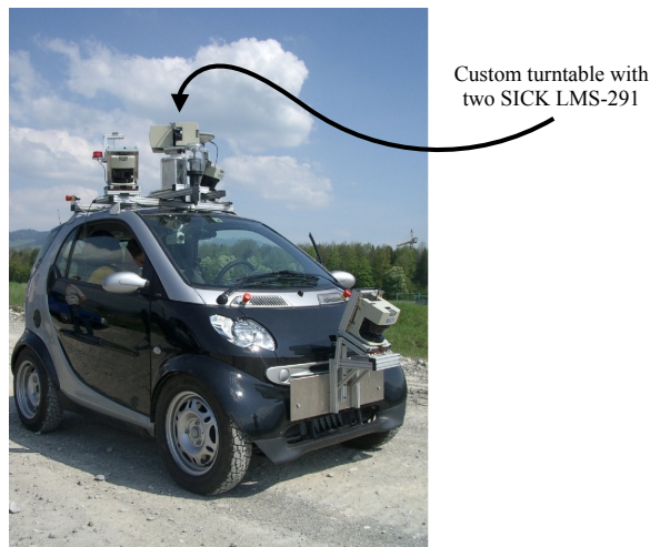
Figure 3.15: The autonomous car, named SmartTer, with its suite of five SICK LMS-291 laser rangefinders. Larger wheels were installed to allow off-road driving.
