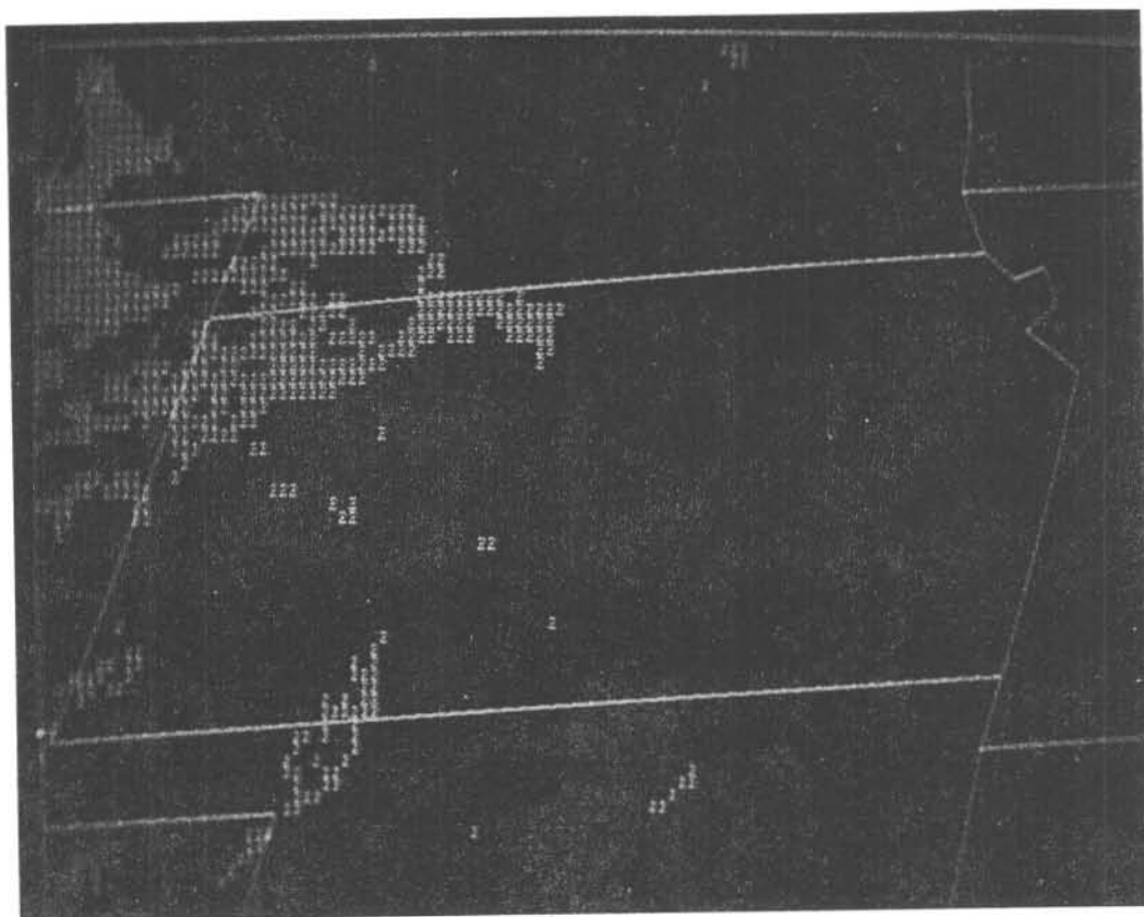
Figure 4. Cloud-top height display from digital IR data taken from GOES-East centered near Wichita, KS, at 2100 GMT of February 7, 1979, as seen on graphics CRT of the AFOS system.
