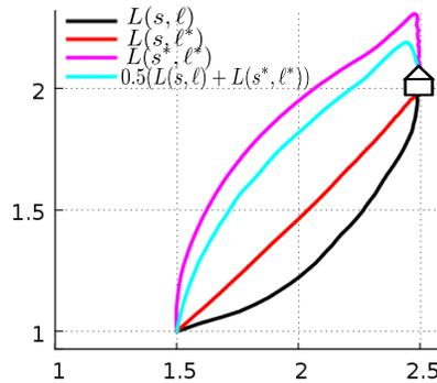
Fig. 5: Homing trajectories with different interaction matrix approximation
