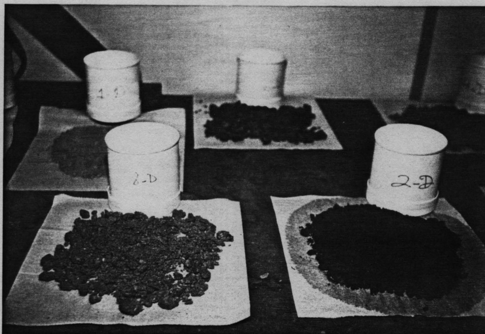
Figure 21. The process of air drying of soil samples was followed by placing them in numbered cardboard containers. (Photograph: Al-Mahawili, 1981)
