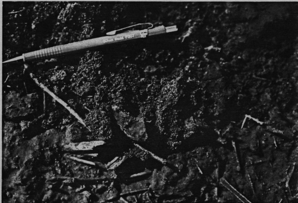
Figure 15. Loose, puffy and white-needle shape features of soils affected by Na_2SO_4 . (Photograph: Al-Mahawili, 1981)
