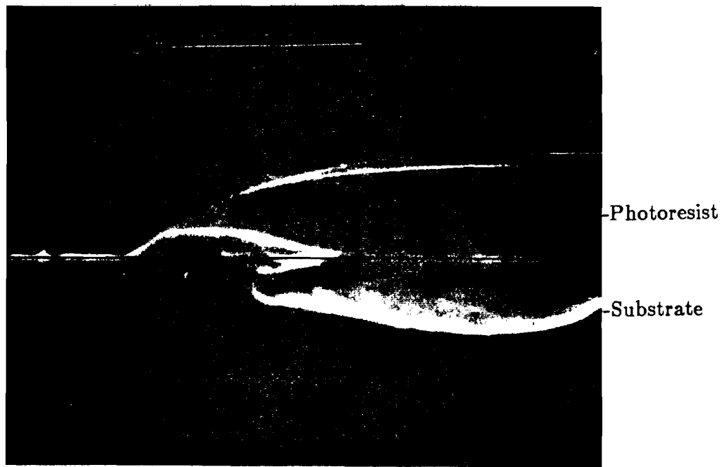
Figure 4.10. SEM cross-section of AZ1350J photoresist sidewall profile processed using standard parameters.
