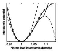
FIG. 1. Schematic interatomic potential used in the Keating (dashed line) and our model (solid line). Dash-dot line plots the potential with the anharmonicity corrections to the VFF constants before the truncation. The line marked with large circles approximatly traces the shape of the realistic potential.
