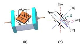
FIG. 1. (Color online) (a) Atomic force microscope image of a 2  $\mu$ m wide Hall bar attached to a piezoelectric. Strain is applied along the [100] and the [010] directions, red dashed lines on the sketch. (b) Hall bar with relative orientation of electrical current  $\vec{I}$ , magnetic field  $\vec{H}$ , and magnetization  $\vec{M}$ .
