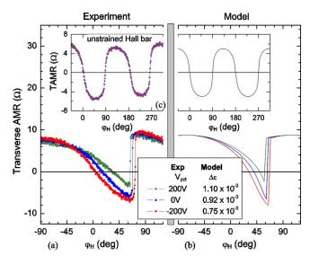
FIG. 2. (Color online) Experimentally measured (a) and modeled (b) transverse AMRs for the strained sample at different voltages on the piezoelectric [data for an unstrained sample are shown in (c)]. All data taken at T=35 K and H=50 mT. The model uses measured strain  $\Delta \varepsilon$ .
