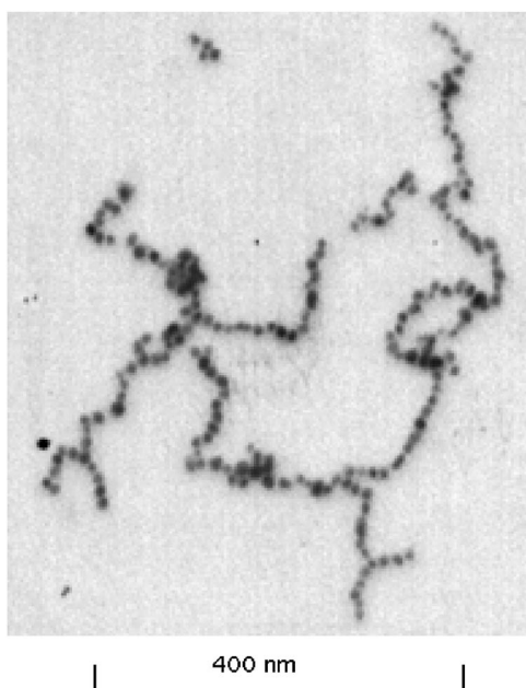
FIG. 1. Transmission electron microscope image of Ag aggregate studied.
