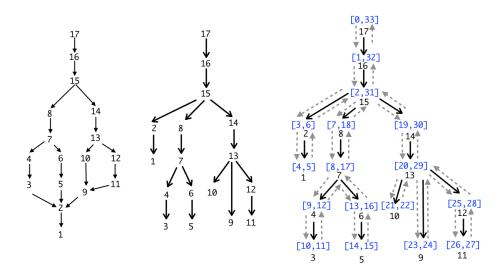
Figure 1. Left: example CFG, with entry point 17, and nodes ordered in reverse postorder (on the left). Center: its dominator tree (where, if i has j as a child, then i is the immediate dominator of j). Right: dominator tree (solid arrows), annotated with a DFS traversal (dotted arrows), and its corresponding DFS intervals (see section 2.3).
