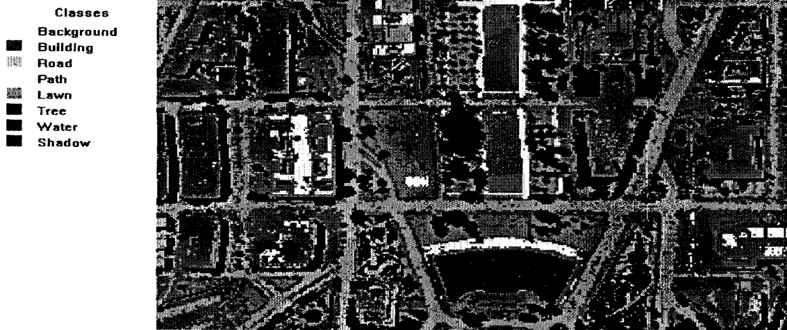
Figure 5.5(c). The thematic map resulting from the classification of the area of Figure 5.4(a) using NWFE features. (In Color)
