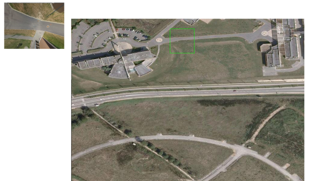
Figure 5: Example of top-down view localization in the aerial image. The top-down view T is the small image on the top left of the Figure, while the green area in the large aerial image A denotes the found localization of T .
