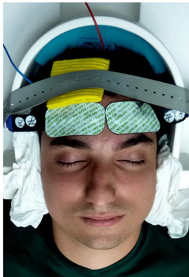
Figure 3.1. SomaSensor based low-cost NIRS data acquisition device to monitor hemodynamics during NIBS.
