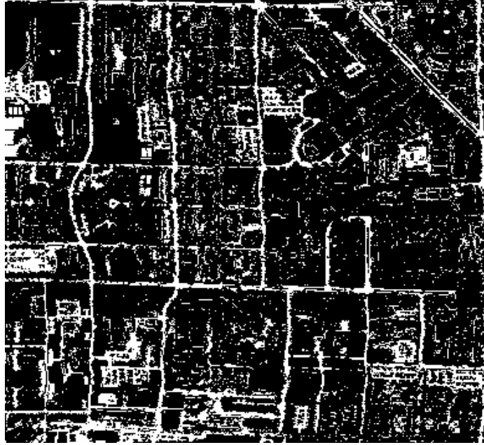
Fig. 4.14 Classification map obtained for “roads and parking lots” in Purdue Campus data during the 1 st iteration of CES 2 C (error=9.0 %)
