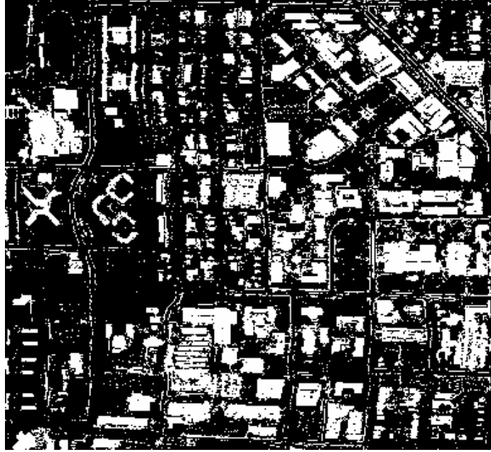
Fig. 4.12 Classification map obtained for “roof tops” in Purdue Campus data during the 20 th iteration of CES 2 C (error=8.3 %)
