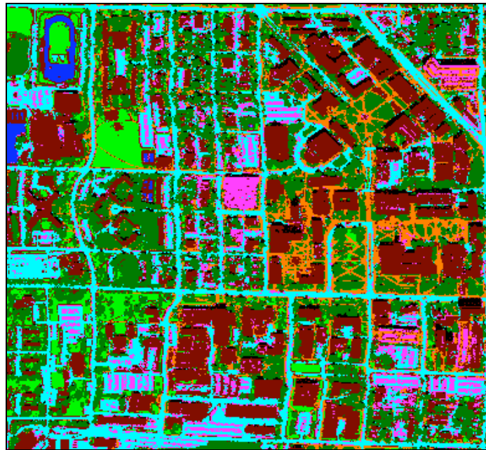
Fig. 2.7 Classification map obtained for the Purdue Campus data by MC for r=0.5 (% error=6.0).
