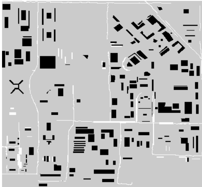
Fig. 4.13 Available ground truth data for “roads and parking lots” in Purdue Campus data (White= roads and parking lots, Black=Not roads and parking lots, Gray= No Assertion)
