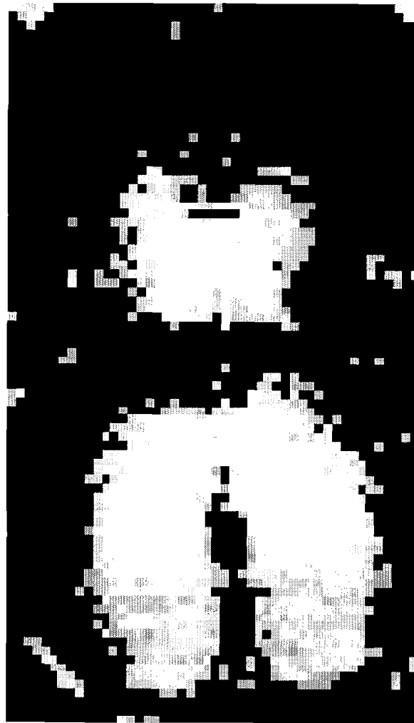
Fig. 2.2. An example of sitting pressure distribution maps displayed as an 8-bit greyscale image. The top half of the image shows the pressure distribution on the back of the chair, and the bottom half shows that of the seatpan. The top, bottom, left and right sides of the image correspond to the shoulder area, knee area, right side and left side of the person, respectively.
