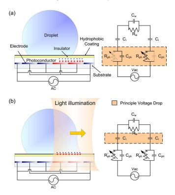
FIG. 2. (Color online) Mechanism of the switching effect for the o-OEW.(a) The liquid droplet maintains a high contact angle and the principle voltage drop falls in the photoconductor in an initial state (without illumination).(b) The impedance of the photoconductor significantly reduces, shifting the voltage drop to the insulator in an excited state (with illumination).
