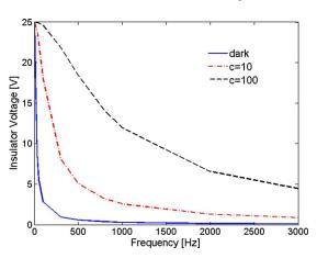
FIG. 3. (Color online) Voltage drop in the insulator vs driving frequency. Notation *c* denotes the photoconductivity ratio (light-to-dark conductivity ratio). The optimal operational region yields the maximum photoconductivity ratio. The driving potential was 50 V<sub>rms</sub> and the empirically operational bandwidth was between 100 and 800 Hz. The frequency out of the range could result in limited or none o-OEW effect.
