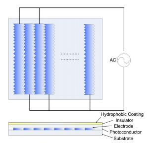
FIG. 1. (Color online) Schematic diagram of the chip layout. The reference and the driving electrodes sit next to each other alternately. The interdigitated edge is used to decrease the discontinuity due to the gap. The materials from the bottom to the top are glass substrate, Ti electrodes, *a*-Si (photoconductor), SiO<sub>2</sub> (insulator), and Teflon (hydrophobic coating).
