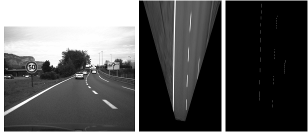
Fig. 10: Ridges detection. (a) Input image. (b) Projected image. (c) Detected ridges.
