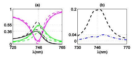
Fig. 3. (Color online) (a) Transmission (black), reflection (magenta) and absorption (green) for a fishnet structure without dye (solid line), with pumped dye molecules in a coating layer (dash-dotted line) and with pumped emitters in coating and spacer layers (dashed line). (b) Reduction in absorption for sample 2 (dash-dotted blue line) and sample 3 (dashed black line).
