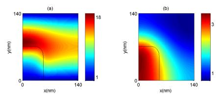
Fig. 5. (Color online) (a) E-field distribution in a quarter unit cell for sample 3 for a cross-section located in the middle of the spacer layer. (b) Same as (a) for a cross-section 15 nm above the fishnet. Here,  $\lambda = 746$  nm.
