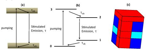
Fig. 1. (Color online) (a) Schematic of stimulated emission from a pumped, broadened two-level system. (b) Same as (a) for a four-level system. (c) Schematic illustration of a quarter unit cell of the fishnet structure studied in simulations. Silver components are shown in blue, spacer layer in light-blue and the gain-composite in red. In some simulations below (sample 3), the gain is also included in the spacer.
