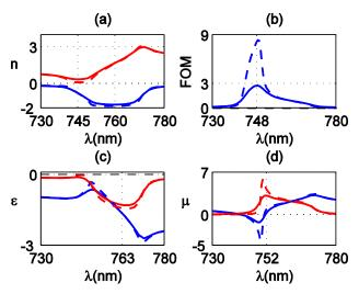
Fig. 4. (Color online) Real parts (blue) and imaginary parts (red) of retrieved effective parameters for samples 1 (solid lines) and 3 (dashed lines).
